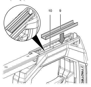
4. Alternatively, the magazine (10) can also be filled with wire nails (8) – insert them on the left-hand side. Observe the mark (11) on the left-hand side of the magazine slider that
