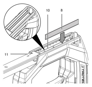
5. Slide the magazine slider (5) back down alongside the magazine (10) until it clicks into place.
